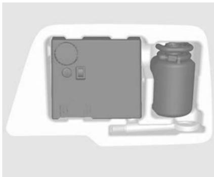
3. Remove the tyre repair kit from behind the cover in the load compartment, on the driver's side.
