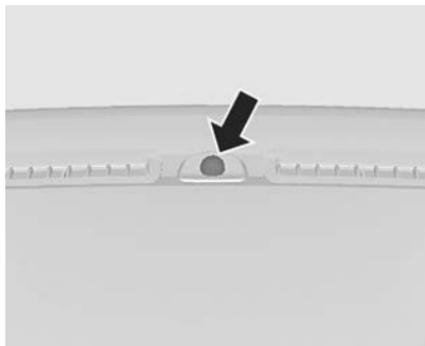
The status LED is located on top of the instrument panel.
