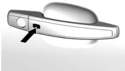
Press the button on the respective door handle. The doors, tailgate and fuel filler door are locked.
