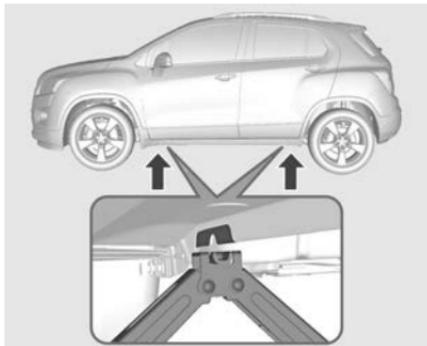
10. Position the jack beneath the jack location closest to the wheel being changed.
