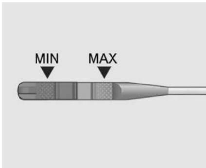
The level should be at the **MAX** mark. Add oil if the level is at the **MIN** mark.
