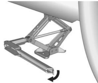
13. Rotate the wrench checking the correct position of the jack, until the wheel is clear of the ground.
