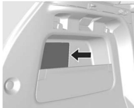
The rear compartment fuse box is located in the passenger's side of the rear compartment.
