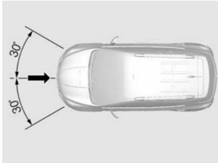
Front airbags will inflate in certain severe frontal or near frontal impacts. Front airbags are not designed to inflate if the vehicle is struck from the side, rear or in rollovers. Always wear a seat belt.
