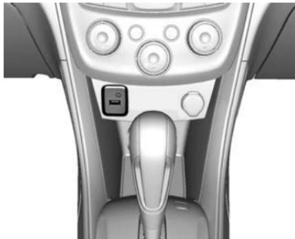
The infotainment system can play the music files contained in a USB storage device, a device that supports Media Transfer Protocol (MTP) or supported iPods/iPhones.
