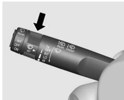
During intermittent operation, adjust the frequency of the wiper intervals:
