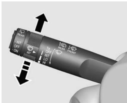
To operate the windscreen wipers, turn the ignition on and move the windscreen wiper/washer lever downwards.
