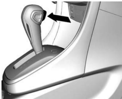
Movement between certain gear positions requires pressing the release button on the shift lever and/or depressing the brake pedal.
