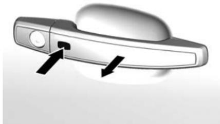
Press the button on the respective door handle and pull the handle. The doors, tailgate and fuel filler door are unlocked.
