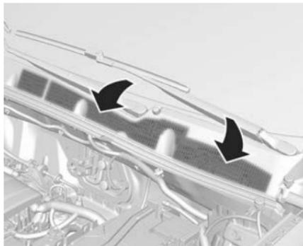
Outside air is drawn into the vehicle through the opening between the bonnet and the windscreen.
