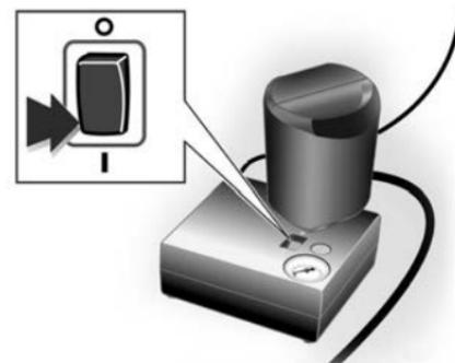
13. Press the switch on the compressor to **I**.
