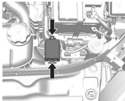
The auxiliary relay box is located in the engine compartment.
