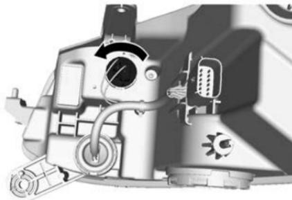
2. Remove the turn signal lamp bulb by rotating anticlockwise.
