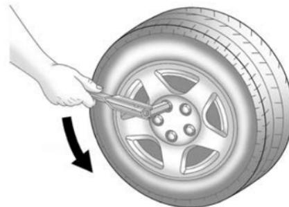
9. Place the wheel wrench over the wheel nuts and loosen by half a turn, but do not remove the wheel nuts.
