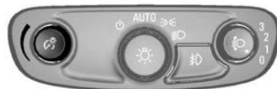
To adjust the instrument panel lighting, press **D** to withdraw the switch, rotate to the desired level and then press it back in place.
