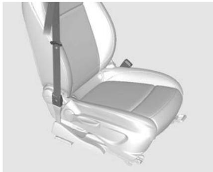
In the event of a front, side or rear collision of a certain severity, the driver's and/or passengers safety belts are tightened.
