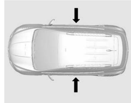
The curtain airbags deploy in most, but not all severe side impacts.
