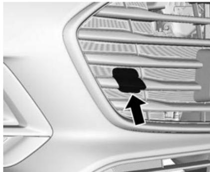
1. Use a screwdriver to disengage and remove the cap.
