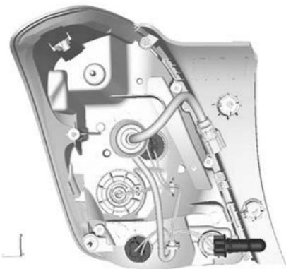
4. Remove the desired bulb holder by rotating anticlockwise.
