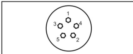
19. With the wheel on the ground, use the wrench to tighten the wheel nuts in the sequence shown.
