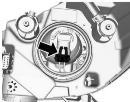
3. Disconnect the wiring harness connector from the bulb.
