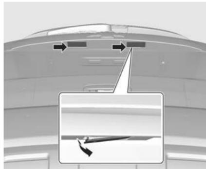
1. Using a flat-blade screwdriver, prise the lamp housing downwards.
