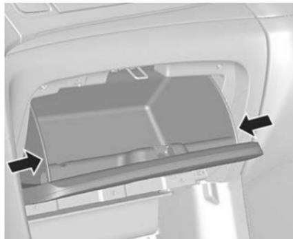
The instrument panel fuse box is located behind the glove box.
