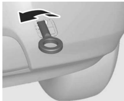
3. Screw in the towing eye anticlockwise until it stops in a horizontal position.
