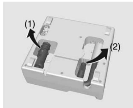
5. Remove the electrical connection cable (1) and air hose (2) from the underside of the compressor.
