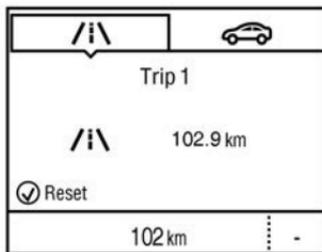
The vehicle has a trip computer displayed on the Driver Information Centre (DIC) in the instrument cluster.
