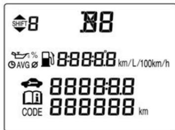
The Driver Information Centre (DIC) is located in the instrument cluster. The DIC may display functions such as the trip computer, information, warning messages and settings, etc.
