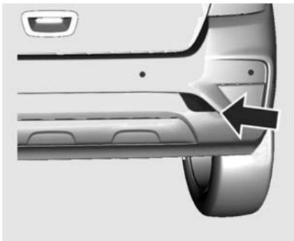
1. Use a screwdriver to carefully disengage and remove the cap.
