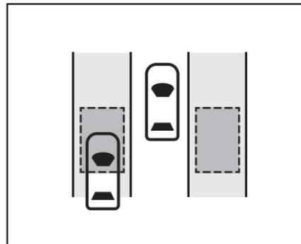
The SBZA sensor covers a zone of approximately one lane over from each side of the vehicle, or 3.5 metres. The height of the zone is approximately between 0.5 metre and 2 metres from the ground.
