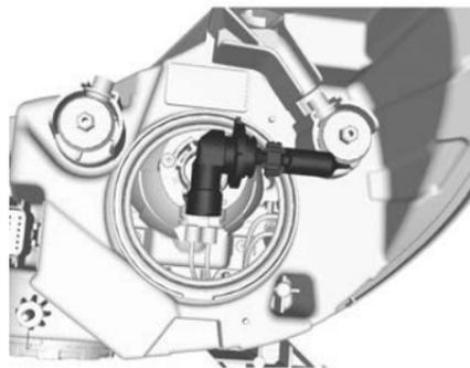
4. Turn the bulb anticlockwise and pull straight back from the headlamp.
