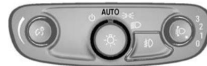
When the lamp control is in the AUTO position, the exterior lamps and instrument panel lights automatically switch on according to ambient light.
