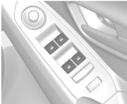
The power windows can be operated when the ignition is turned on.
