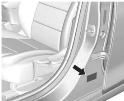
An identification label is located on the lower portion of the front passenger's door frame.
