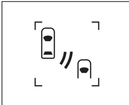
When the engine is started, both outside mirror SBZA displays will briefly illuminate to indicate the system is operating.
