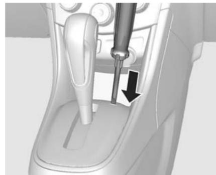
7. Press the screwdriver into the slot. The ignition key can if a screwdriver is not available.
