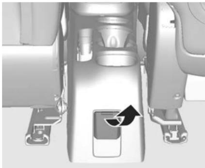
A 230V power outlet is located at the rear of the centre console.
