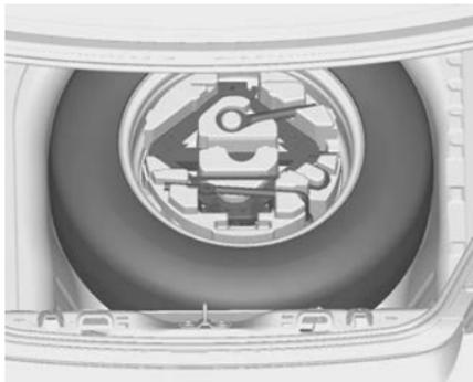
The jack and tools are located above the spare wheel, in the load compartment.
