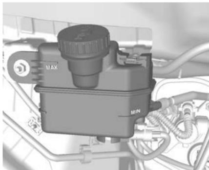
The level should be between the **MIN** and **MAX** area.
