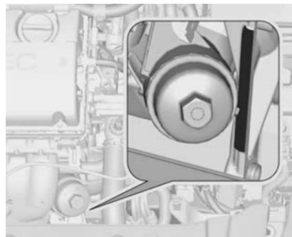
The engine serial number is located next to the oil filter.
