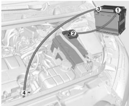
6. Connect one end of the RED lead to the positive terminal of the booster battery (1).
