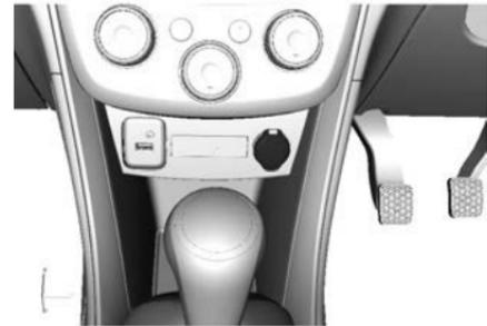
A 12V power outlet is located in the centre console.
