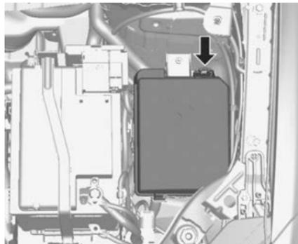
The fuse box is located in the engine compartment.
