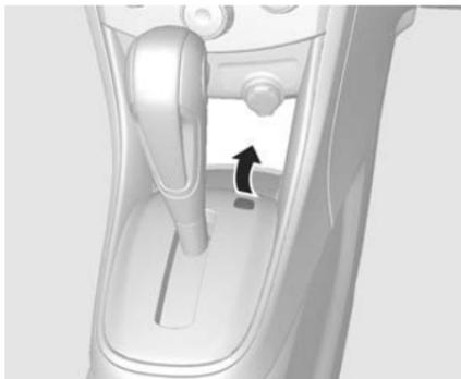
6. Remove the cap on the centre console with a thin object such as a flat-blade screwdriver.
