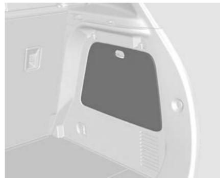
The tools and tyre repair kit are located in the load compartment on the driver's side.
