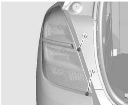
2. Disengage the two screw covers and remove the two screws securing the tail lamp assembly.
