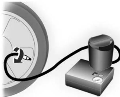
11. Unscrew the valve cap from the defective tyre.
