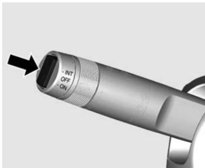
To operate the rear window wiper, push the switch at the end of the lever.
