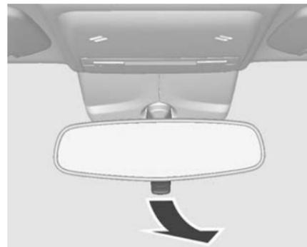
To reduce headlamp glare from following vehicles, pull the lever towards the rear of the vehicle.
