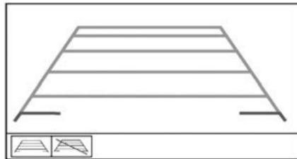
When the camera image is displayed, dynamic guidelines are also displayed to assist with reversing the vehicle.
