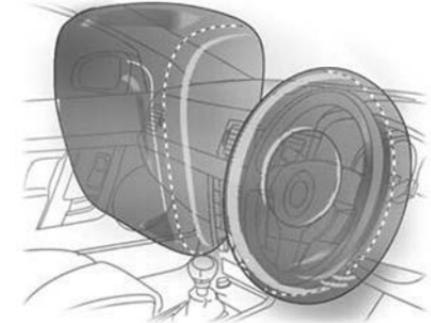
The front airbag system consists of one airbag in the steering wheel and one in the instrument panel on the passenger's side. These are identified by the word **AIRBAG**.
