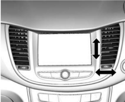
Centre air vent volume may be controlled by turning the adjuster wheel under the vent.
