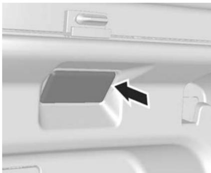
1. Using a flat-blade screwdriver, prise the lamp assembly outwards.
