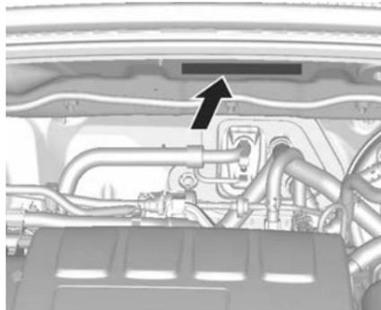
The Vehicle Identification Number (VIN), is engraved in the centre of the firewall and also on a plate on the passenger's side at the lower edge of the front windscreen.
