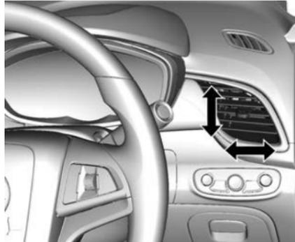
Side air vent air flow may be closed by sliding the vent adjuster fully outboard.
