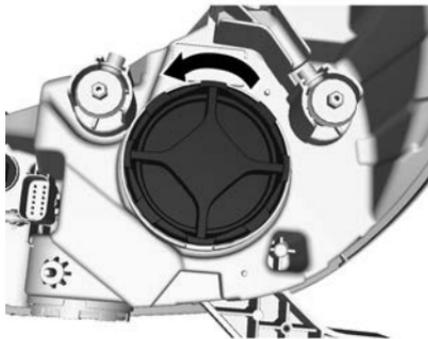
2. Remove the headlamp bulb cover by rotating anticlockwise.
