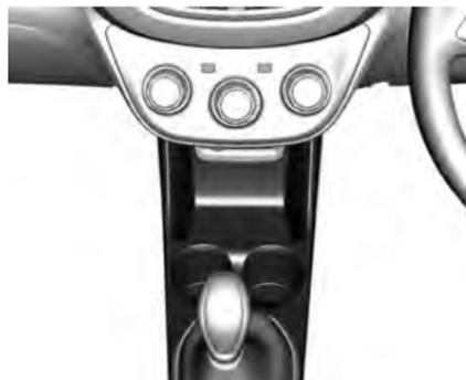
The instrument panel storage compartment is located in front of the shift lever.
