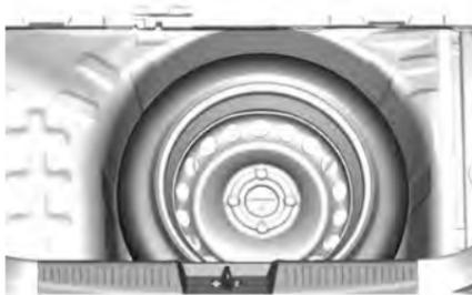
The spare tyre is located in the load compartment beneath the floor covering.
