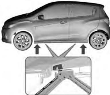
14. Position the jack beneath the jack location closest to the wheel being changed.
