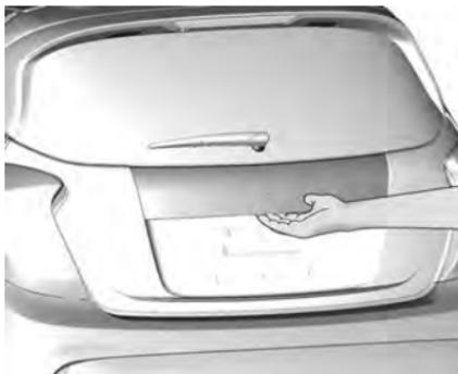
To open the tailgate, with all doors unlocked, press the touchpad switch on the underside of the tailgate moulding and lift up.
