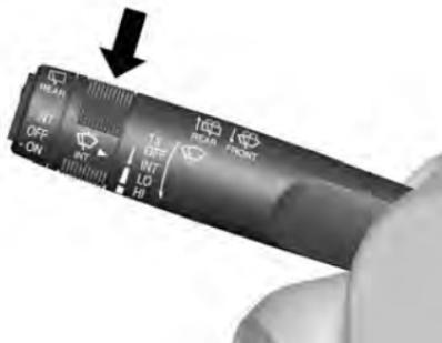
During intermittent operation, adjust the wiper interval:
