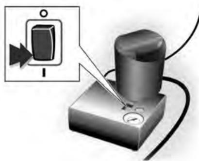
15. Press the switch on the compressor to I.
