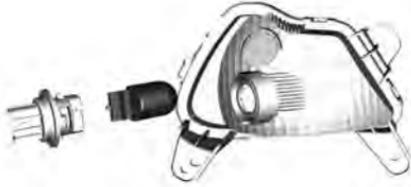
2. Disconnect the electrical connector from the bulb holder.
