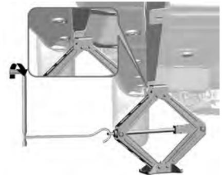
Ensure the jack is not tilted and the base is resting squarely on the ground.
