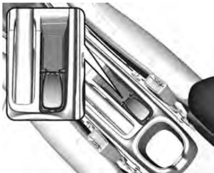
Place the electronic key in the centre console transmitter pocket. Press the brake pedal and press the Engine Start/Stop button.
