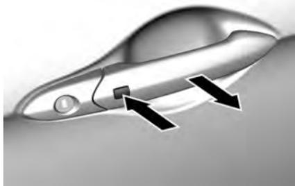
Press the button on either front door handle. The doors and tailgate are unlocked.
