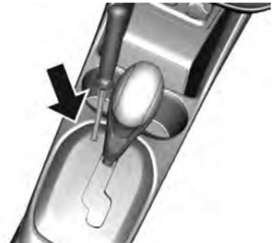
3. Insert a flat-blade screwdriver into the opening as far as it will go and move the shift lever out of P (park).
