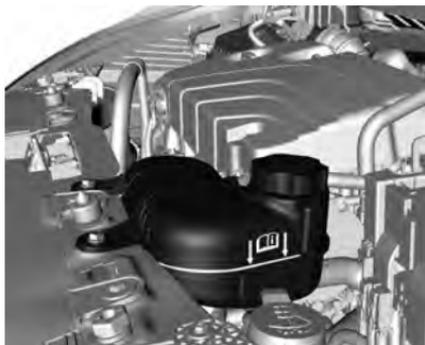
If the cooling system is cold, the coolant level should be above the line on the coolant reservoir.
