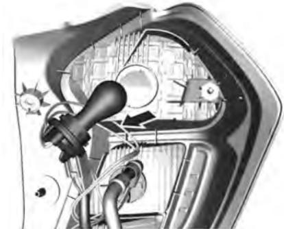
4. Push the bulb into the socket slightly and rotate anticlockwise to remove.
