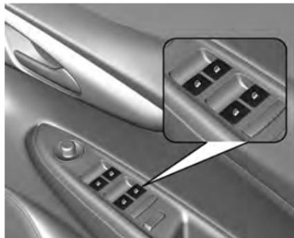
The power windows can be operated when the ignition is on.
