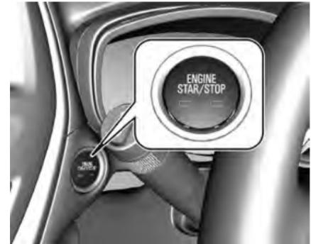
Electronic key must be inside the vehicle.
