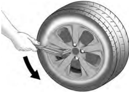
13. Place the wheel wrench over the wheel nuts and loosen by half a turn, but do not remove the wheel nuts.
