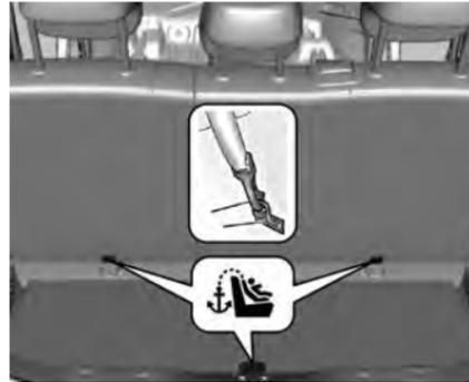
The child restraint tether anchors are located on the backside of the rear seats and the centre of the rear end panel at the load compartment area.
