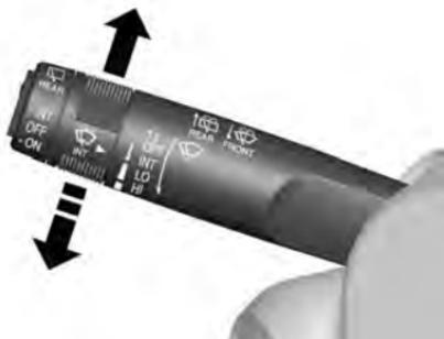
To operate the windscreen wipers, turn the ignition on and move the windscreen wiper/washer lever up or down to the desired position.
