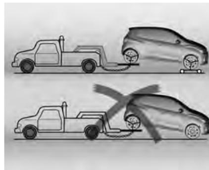
2. Alternatively, use a standard tow truck and a towing dolly to prevent the front wheels from contacting the road.
