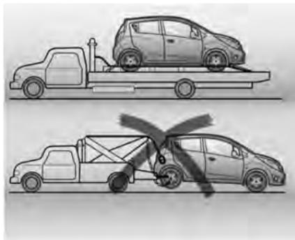
A flat-bed tow truck is the best method of towing the vehicle to avoid damage.
