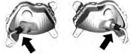
7. Reconnect the electrical connector and ensure the locking pin is placed correctly.
