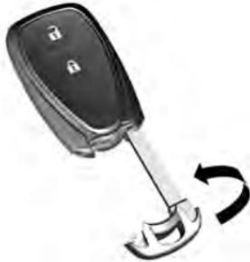
1. Press button on the side of the transmitter to remove the key blade.
