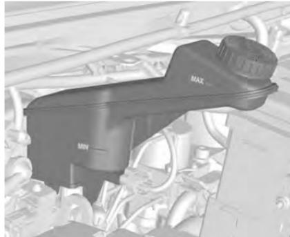
Check the brake fluid level weekly. The level should be between the **MIN** and **MAX** area.
