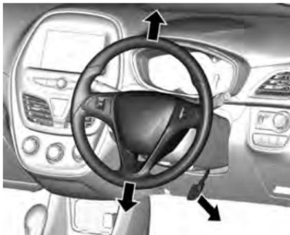
1. To unlock, move the lever down.
