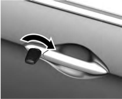
1. Insert the key into the driver's door by turning the key towards the front of the vehicle.
