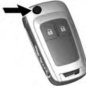
1. Press the button to extend the key blade.
