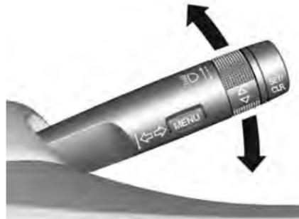
1. Push the lever in the direction the steering wheel is turned.
