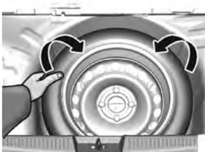
11. Remove the spare wheel from the load compartment:
