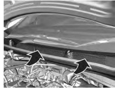
Outside air is drawn into the vehicle through the opening between the bonnet and the windscreen.
