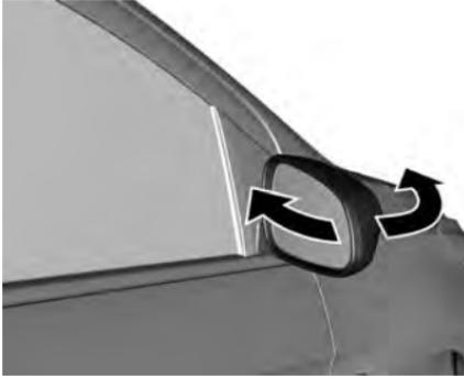
When the vehicle is parked, the mirrors may be folded flat against the side of the vehicle.
