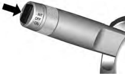
To operate the rear window wiper, push the switch at the end of the lever.
