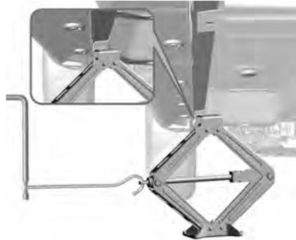
16. Attach the jack handle to the jack and attach the wheel wrench to the jack handle.
