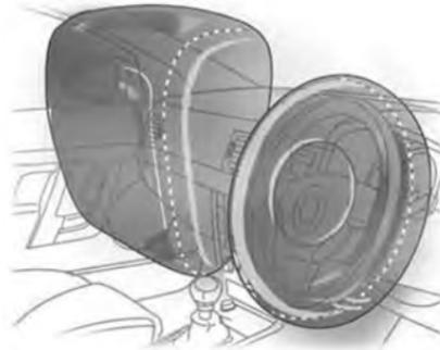
The front airbag system consists of one airbag in the steering wheel and one in the instrument panel on the passenger side. These are identified by the word AIRBAG.
