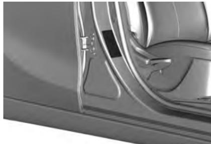
The correct pressures for tyres are shown on the tyre placard in the driver's door frame and in the tyre pressure table.
