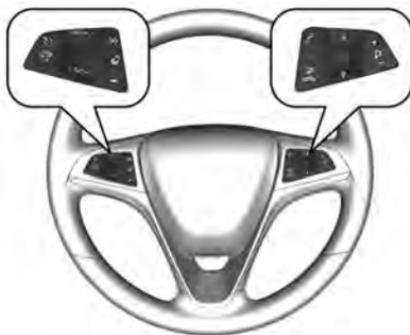
The infotainment system and the cruise control may be operated by the controls on the steering wheel.
