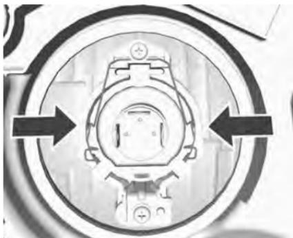
7. Press the spring clip to disengage.
