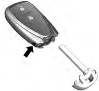
Press button on the side of the transmitter to remove the key blade.
