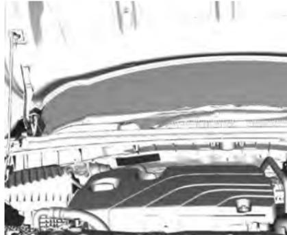
The vehicle identification number (VIN) is stamped in the engine compartment panel and is also located behind the windscreen on the passenger side.
