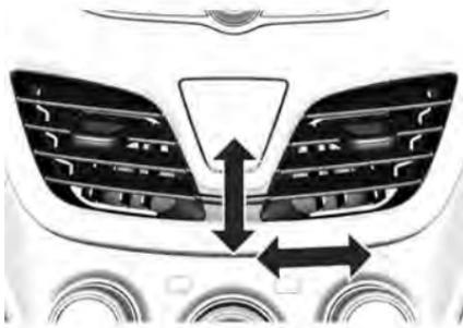
Direct the air flow by tilting and swivelling the slats.
