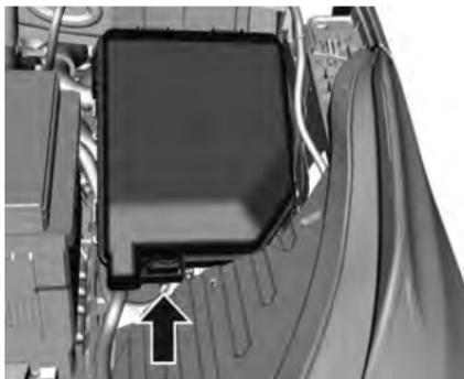
1. To disengage the cover, lift upwards and remove.
