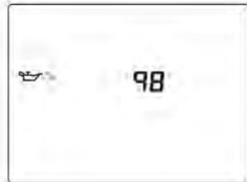
Displays an estimate of the remaining useful oil life. This may only be displayed while the vehicle is stationary.
