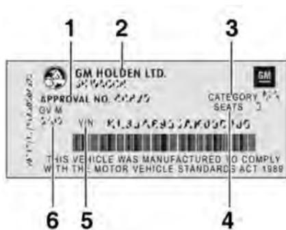
An identification and compliance label is located on the front passenger door frame.
