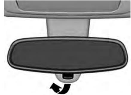
To reduce headlamp glare from following vehicles, push the lever towards the front of the vehicle.
