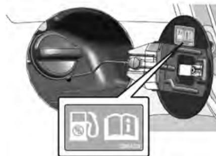
4. Remove the cap. The cap is tethered to the vehicle.
