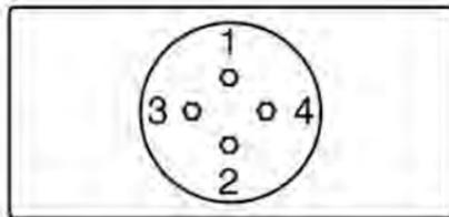
24. With the wheel on the ground, use the wheel nut wrench to tighten the wheel nuts in the sequence shown.
