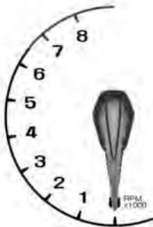
Shows engine speed in thousands of revolutions per minute (RPM).
