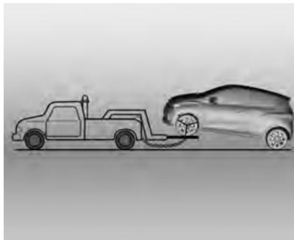
1. Use a standard tow truck, where the front wheels are raised and the rear wheels are in contact with the ground.
