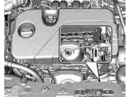
The engine serial number is located in the front part of the engine compartment.
