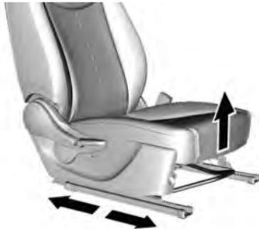
1. Move the seat forwards or backwards by lifting the bar at the front and sliding the seat.
