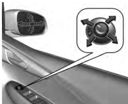
Select the relevant exterior mirror by turning the control left (L) or right (R). Then swivel the control to adjust the mirror.
