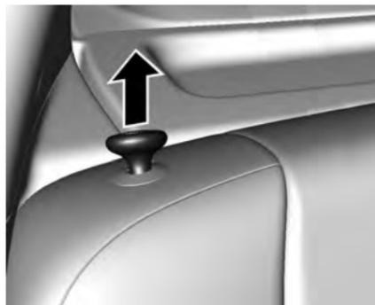
6. Pull the release knob on top of the rear seatback upwards.
