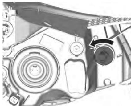
1. Rotate the bulb holder anticlockwise to disengage.
