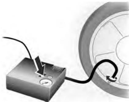
27. Screw the compressor air hose directly onto the tyre valve and compressor to check the tyre pressure.
