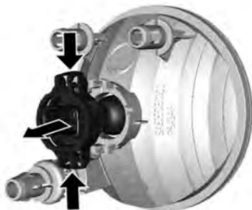
2. Disconnect the electrical connector from the bulb holder.
