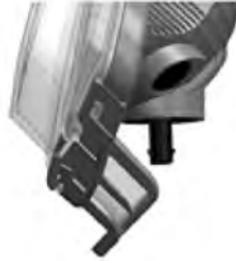
6. Reinstall the bulb holder into the lamp and rotate it clockwise until the centre of the bulb holder is placed at the arrow shape on the lamp.
