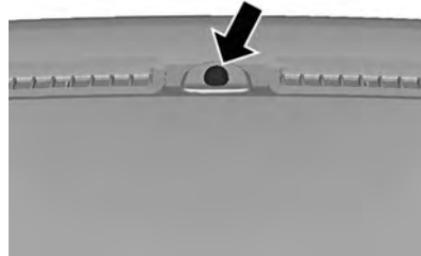
A status LED is integrated in the sensor on top of the instrument panel.
