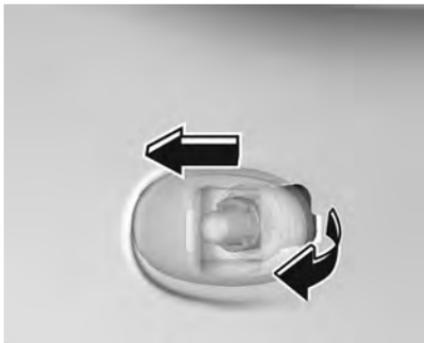
1. Push the lamp towards the front of the vehicle and remove.
