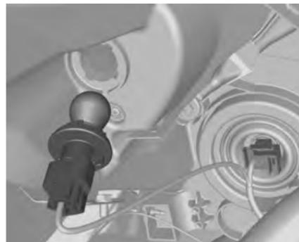
2. Push the bulb into the socket slightly and rotate anticlockwise to remove.
