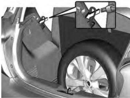
3. Place the loop end of the strap through the seatback latch.
