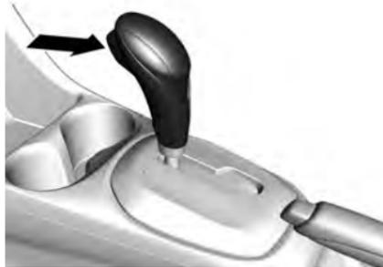
Movement between certain gear positions requires pressing the release button on the front of the shift lever.
