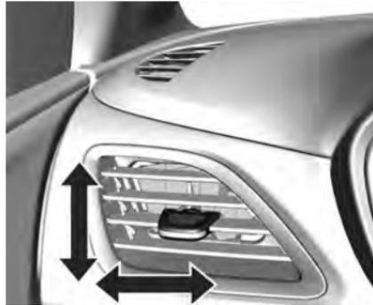
Direct the air flow by tilting and swivelling the slats.
