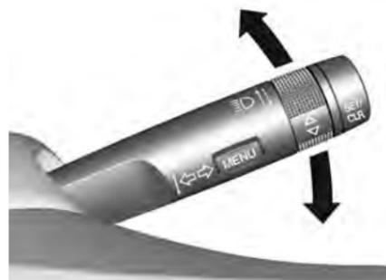
Push the lever in the direction the steering wheel is turned.
