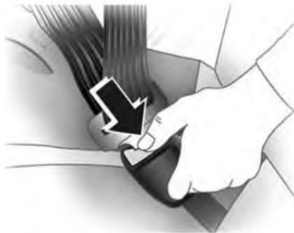
1. Press the release button on the buckle.
