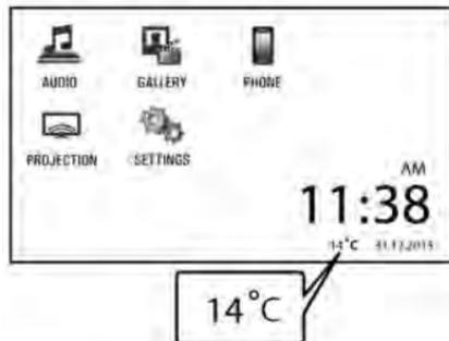
The outside temperature is shown in the infotainment display when the ignition is on.
