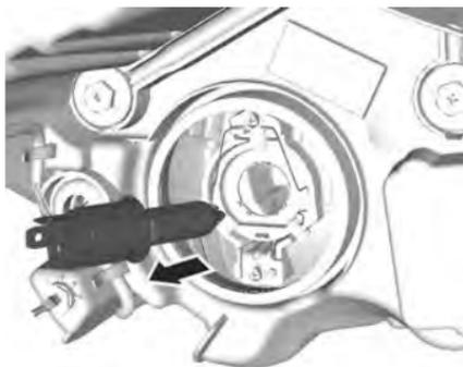
8. Remove the bulb from the reflector housing.
