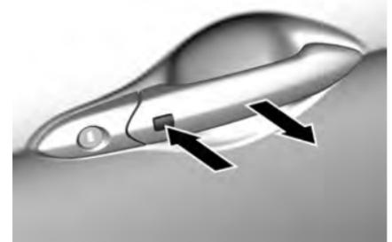
Electronic key system: Unlocking the vehicle by pressing the button on a front door handle deactivates the anti-theft system.
