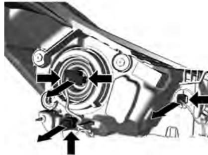
4. Push the retaining tab and then remove the electric connectors from the headlamp.
