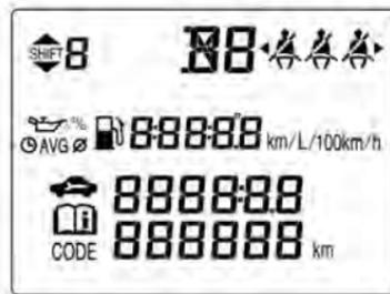
The Driver Information Centre (DIC) is located in the instrument cluster. The DIC displays functions such as the trip computer, information and warning messages and settings, etc.
