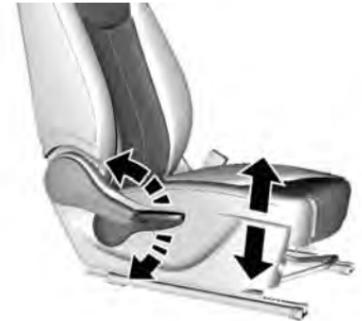
Pump the lever on the outside of the seat cushion.
