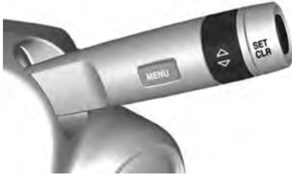
Rotate the adjuster wheel
