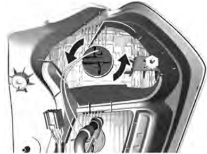
3. Rotate the applicable bulb holder anticlockwise.
