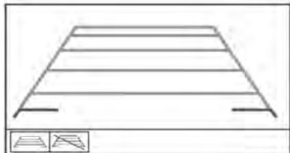
When the camera image is displayed, static guidelines are also displayed to assist with reversing the vehicle.
