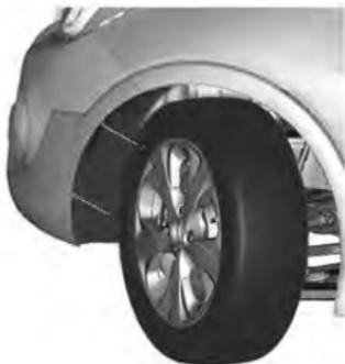
1. Turn the front wheels and remove 2 push nuts on outside of wheel liner.
