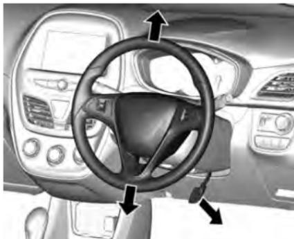
1. To unlock, move the lever down.
