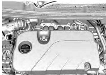
1. Rotate the engine oil filler cap anticlockwise and remove.
