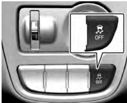
TCS can be switched off when spinning of drive wheels is required:
