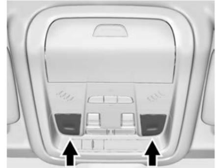
Press the lamp lenses to manually turn the front reading lamps on or off.
