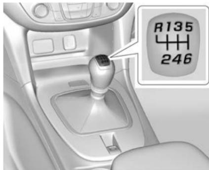
The manual transmission has six forward gears and a reverse gear.
