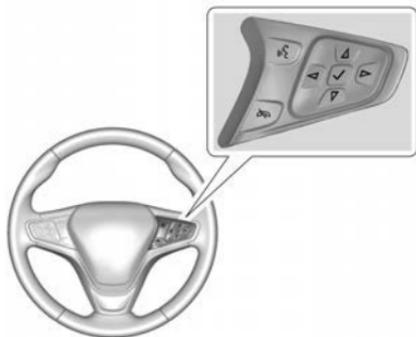
Some of the audio controls can be adjusted on the steering wheel.
