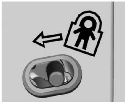
The rear door child safety locks prevent passengers from opening the rear doors from inside the vehicle.
