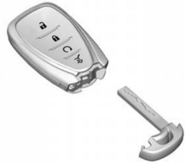
1. Press the button on the side of the RKE transmitter and remove the mechanical key.
