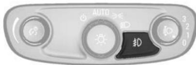
The fog lamps button is on the instrument panel beside the steering wheel.
