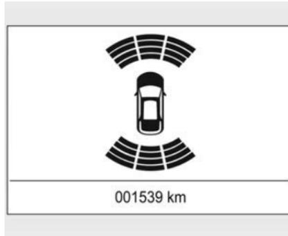
Additionally, the distance to rear and front obstacles is displayed by changing distance lines in the DIC.
