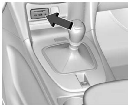
The front USB port is located at the front of the centre console, below the climate control system. It contains an A-type and a C-type USB outlet.
