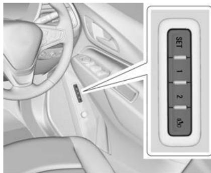
If equipped, memory seats allow two drivers to store and recall their unique seat positions for driving the vehicle, and a shared exit position for getting out of the vehicle. For seat entry memory recalls, the positions are linked to both RKE transmitters.
