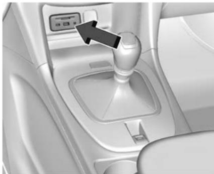
The vehicle has a USB port with an A-type and a C-type USB outlet located at the front of the centre console. These outlets are for data and charging. A USB port with one or two A-type USB outlets may also be fitted at the rear of the centre console for charging only.
