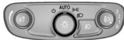
The exterior lamp control is located on the instrument panel on the outboard side of the steering column.
