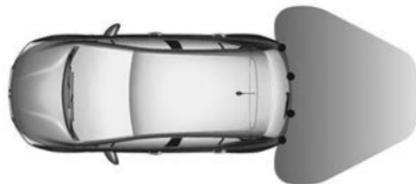
The system uses ultrasonic parking sensors located in the rear bumper.
