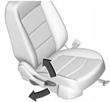
Move the lever up or down to manually raise or lower the seat.
