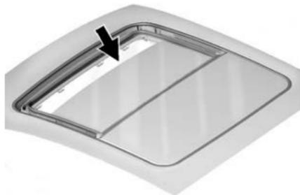
Dirt and debris may collect on the sunroof seal or in the track. This could cause an issue with sunroof operation or noise. It could also block the water drainage system. Periodically open the sunroof and remove any obstacles or loose debris. Wipe the sunroof seal and roof sealing area using a clean cloth, mild soap, and water. Do not remove grease from the sunroof.
