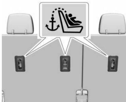
Top tether anchors are located on the back of the rear seat backs and are identified with symbol
