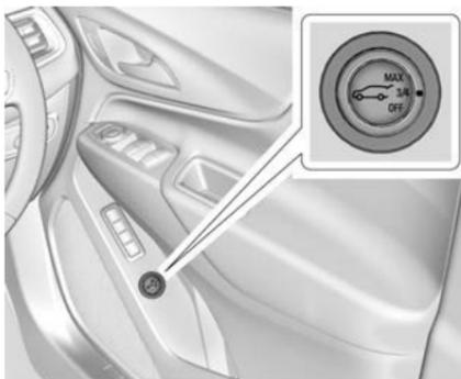
Choose the power liftgate mode by turning the dial on the switch to either the 3/4 or MAX position.
