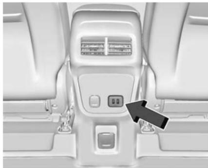
A USB port may also be located at the rear of the centre console. This port is for charging USB devices only.
