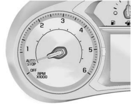
An Auto Stop is indicated by the tachometer needle moving to the AUTO STOP position. Once the engine restarts, the engine speed indication is resumed.
