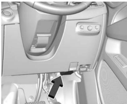
The instrument panel fuse panel is located under the instrument panel on the driver side.
