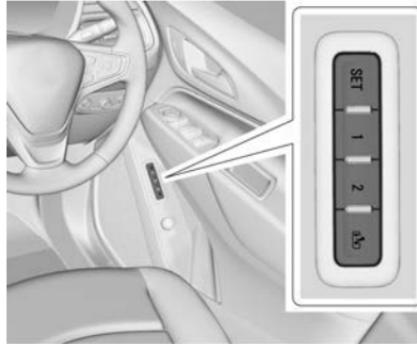
If equipped, the memory seat function allows two drivers to save and recall their unique seat position for driving the vehicle, and a shared exit position for getting out of the vehicle.
