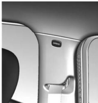
Curtain airbags are stored in the roof on each side of the vehicle.
