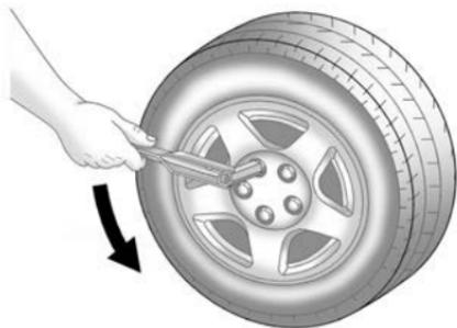
8. Turn the wheel wrench anticlockwise to loosen all the wheel nuts. Do not remove them yet.
