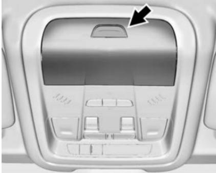
A covered storage compartment for sunglasses is located in the overhead console. Press the latch to open.
