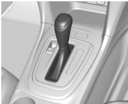
Press the select button on the front of the shift lever to move into any position. The lever position is displayed in the Driver Information Centre (DIC).
