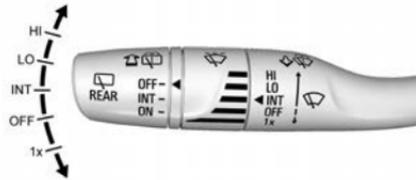
With the ignition on or in Accessory mode, move the windscreen wiper lever to select the wiper speed.
