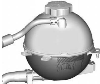
Check the coolant level in the coolant surge tank when the engine is cold.
