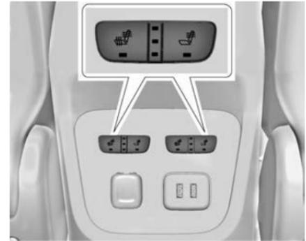
If equipped, the rear heated seat controls are on the rear of the centre console. To operate, the engine must be running.
