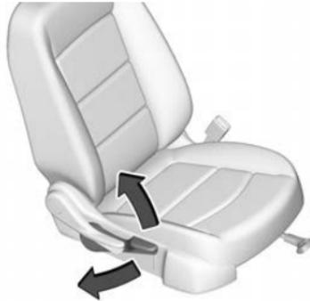
Move the lever up or down to raise or lower the seat.
