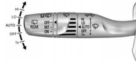
With the ignition on or in Accessory mode, move the windscreen wiper lever to select the wiper speed.
