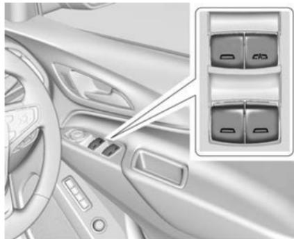
Power windows can be operated when the ignition is on, in Accessory mode, or when Retained Accessory Power (RAP) is active. See *Retained Accessory Power (RAP)* ⇨ 194.
