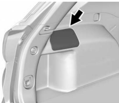
To access the fuse panel, carefully release the upper edge and remove the trim plate.
