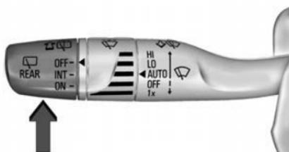
Turn the end of the windshield wiper lever to operate the rear window wiper/washer.
