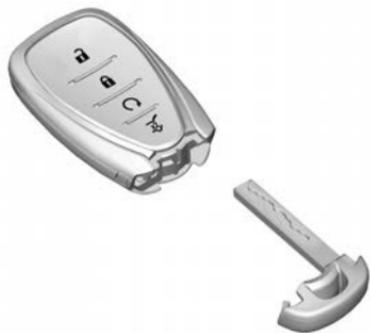
Remove the mechanical key by pressing the button on the side of the RKE transmitter near the bottom and pull the key out. Never pull the key out without pressing the button.
