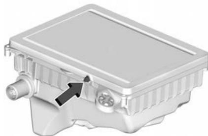
1. Align the air cleaner/filter with the indicated point on the base of the air cleaner/filter housing and install the air cleaner/filter. The outer air cleaner/filter seal must be fitted properly in the air cleaner/filter housing.
