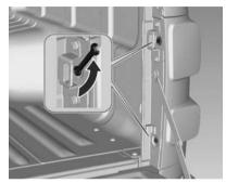
1. Unscrew both fasteners.
