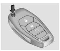
Press the button to extend the key blade. To retract the key blade, press the button and fold the blade into the key.
