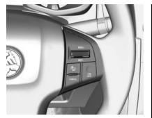
The Cruise Control and the Forward Collision Alert can be operated by the controls on the steering wheel.
