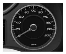
Shows vehicle speed in kilometres per hour (km/h).
