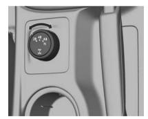
Rotate the transfer shift control switch to change the setting.
