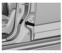
A label containing the vehicle build date is also located on the front passenger's door frame or on the rear door frame (Space Cab).
