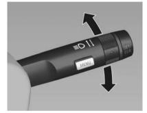
Push the lever in the direction the steering wheel is turned.
