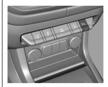
The P™ button on the instrument panel is used to turn on or off the front and rear parking assist. The indicator next to the button illuminates when the features are on and turns off when the features have been disabled.
