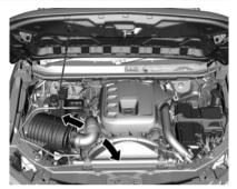
Remove the support rod from the holder and secure in the bonnet aperture.
