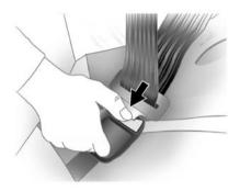
To release the belt, press the red button on the belt buckle.
