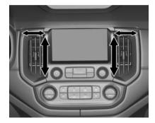
Push the adjuster knob up to open and down to close the vent or to adjust the volume of air.
