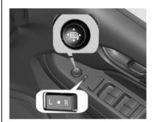
The controls for the power mirrors are located on the driver's door.
