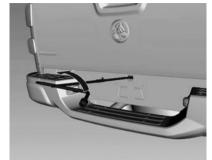
Rotate the wheel wrench anticlockwise to lower the spare tyre to the ground.
