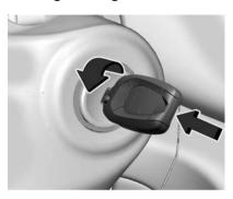
When the vehicle is stopped, push the key in toward the steering column and turn the key to Lock / Off to turn the engine off.
