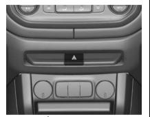
Press to turn the hazard warning flasher on or off, when the ignition is in any position.
