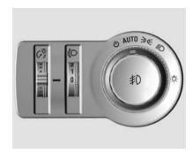
ウ: With automatic headlamp system, turn the switch to activate or deactivate the system. The switch returns to **AUTO**.
