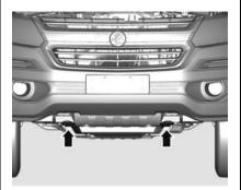
The vehicle may be recovered using the front towing eyes.
