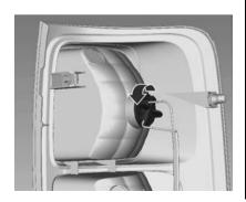
4. Rotate the relevant bulb holder anticlockwise.
