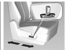
Move the seat forwards or backwards by sliding the switch.
