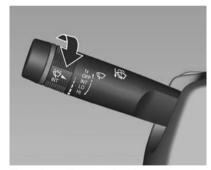
Turn the adjuster wheel to adjust the sensitivity:
