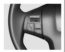
The infotainment system can be operated by the controls on the steering wheel.
