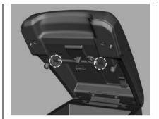
Use the recesses as shown to prevent the cable from being pinched when the armrest is closed.
