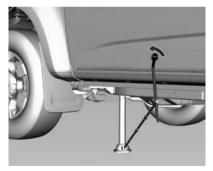
If the flat tyre is on the front of the vehicle, position the jack under the chassis rail between the two braces as shown (1).
