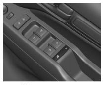
Press to deactivate the rear door power window switches. The rear door power windows can still be operated by the driver's door switches.
