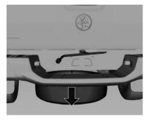
Continue to rotate the wheel wrench until the spare tyre can be pulled out from under the vehicle.
