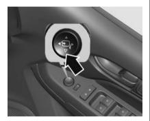
Press the selector switch (L / R switch) to the central position •, then push the four-way switch down Both exterior mirrors will fold
