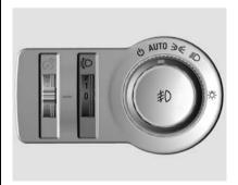
To set the headlamp level according to vehicle load, turn the dial to the required position.
