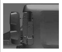
Remove the tail lamp assembly by pulling it straight out from the body. Take care that the cable duct remains in position.
