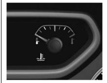
Shows the engine coolant temperature.
