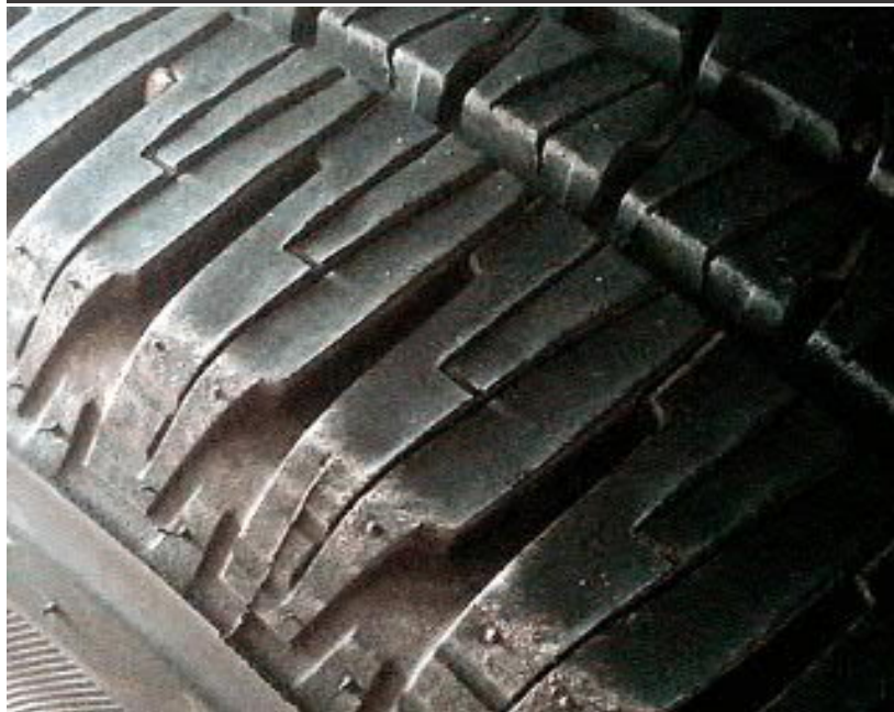
Figure 3: Tyre Shoulder View Example 2 - "NORMAL" Tyre "Feathering" Wear
